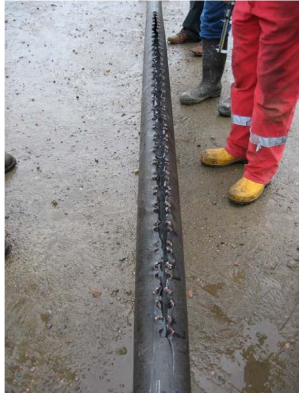
Fig. 6. Joint of 4 1/2-in. Tubing Shot with Two Guns
