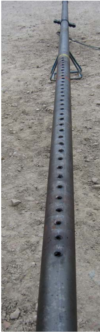
Fig. 5. Joint of 4 1/2-in. Tubing Shot with One Gun
