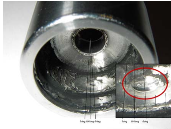
Fig. 16. Orientation Confirmation Device Showing Actual Orientation of the Gun Downhole When Fired
